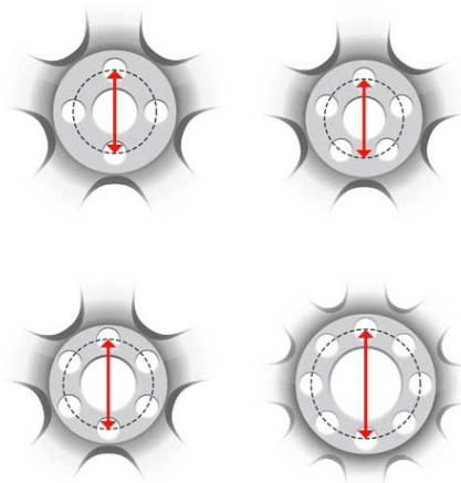
The bolt pattern of the replacement wheels must match that of the vehicle. The bolt pattern is often stamped on the wheel or the wheel box.
