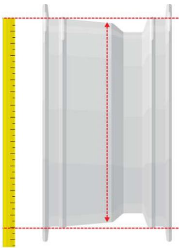
In Wheel Basics we learned about how tires and wheels of different diameters are not compatible and could result in bead failure during inflation. The diameter of the tires and wheels must match exactly!
