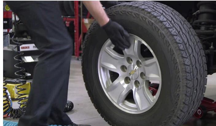
Be sure to clean the wheel and hub before proceeding with the test fit.
