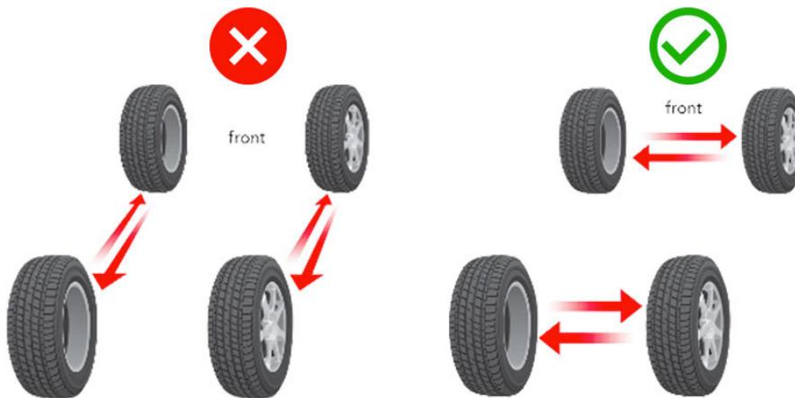
If you find the service instructions on the work order do not meet the requirements of a staggered vehicle (ex: front to back rotation), notify the Salesperson before beginning service.
