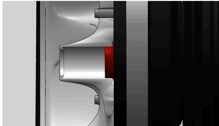
Place a bare wheel on the hub and check for interference against the brake calipers, hub, or suspension components. If the wheel sits flush against the hub, it should be turned by hand 360° to ensure no low spots make contact. Never turn or spin a wheel by handling the spokes or inner barrel of the wheel.
