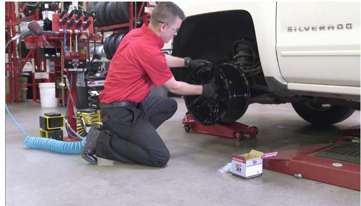
Following the bare wheel and lug nut checks, mount the tire on one wheel and install the assembly on the vehicle.
