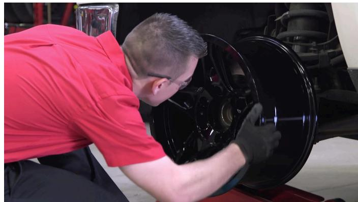
Next come the lug nuts. This involves verifying the thread engagement and lug seat. Make sure the seat of the wheel and the lug nut match.
