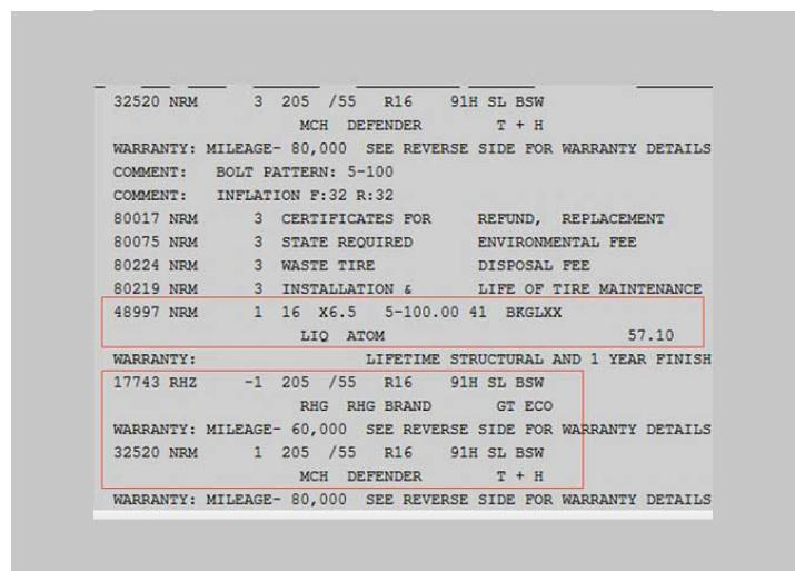
During a pre-service vehicle inspection, make sure the tire's rim diameter matches the wheel's diameter. If they do not match, notify the Salesperson immediately.
