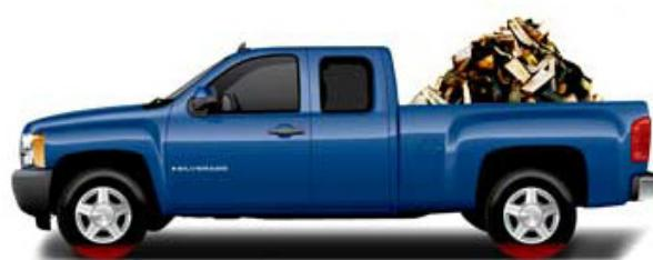
The load index of the replacement tire must meet or exceed the Reserve Load for the vehicle. The Reserve Load is defined by the load carrying capacity of the OE tire load index at the OE cold inflation pressure.
