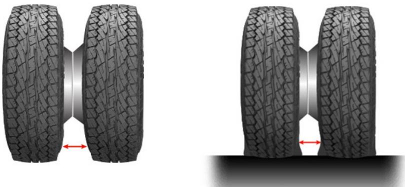
Tire sidewalls bulge slightly more where they meet the road. At this point, dual wheel tires must not come into contact with each other, as this rubbing may cause damage to both tires. This is usually the sign of a section width versus rim width issue.
