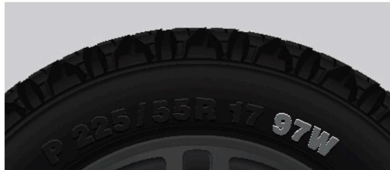
The speed rating is a letter indicating the maximum speed that a tire can safely reach and maintain, as determined by laboratory testing.
