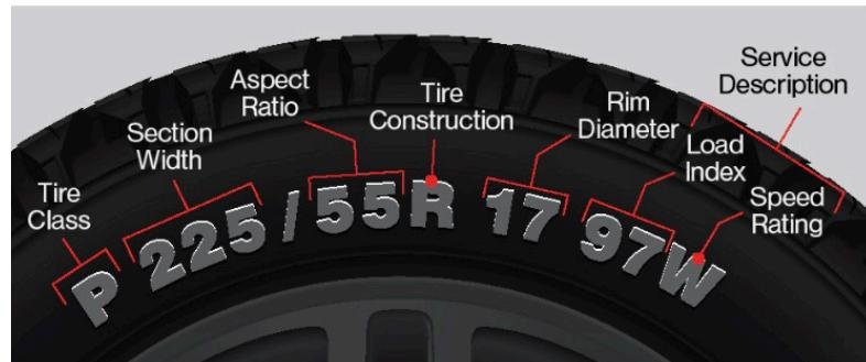
The first number represents the **section width** in millimeters.
