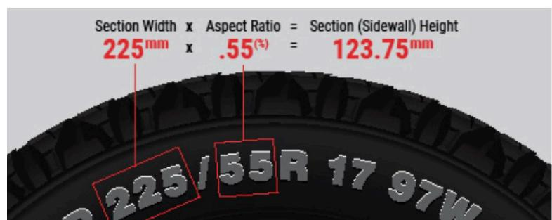
Last is the **rim diameter**, which indicates the diameter of the wheel on which the tire can be mounted.
