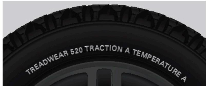
The **traction grade** appears next. This ranking describes the tire's ability to stop on straight, wet surfaces under controlled conditions.
