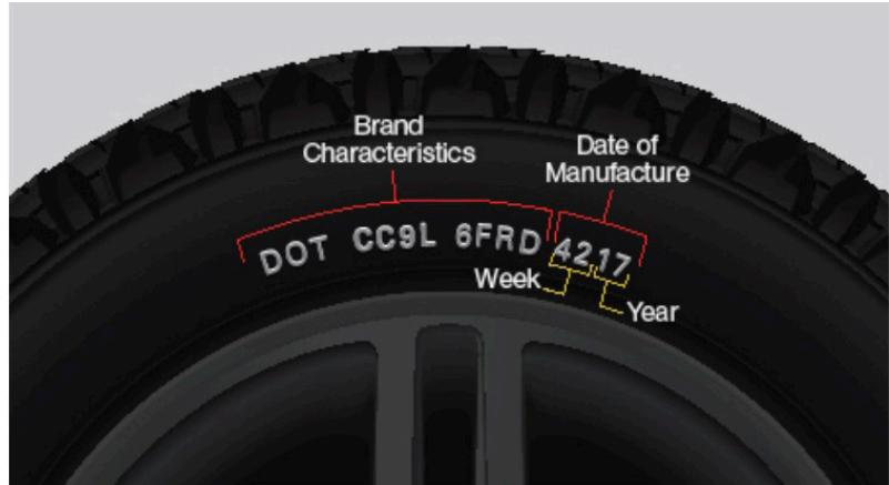
The most important information are the last three or four numbers after the brand characteristics. These numbers represent the date that the tire was manufactured. If the tire was manufactured after the year 2000, you will find four numbers.
