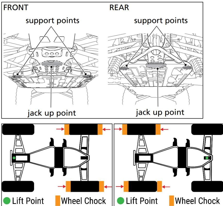
Because you must raise the vehicle by the center, you will only be able to raise either the front or the rear of the ATV/UTV at one time. When raising an ATV/UTV, place wheel chocks in front of and behind the assemblies on the axle opposite of the one that is being raised.
