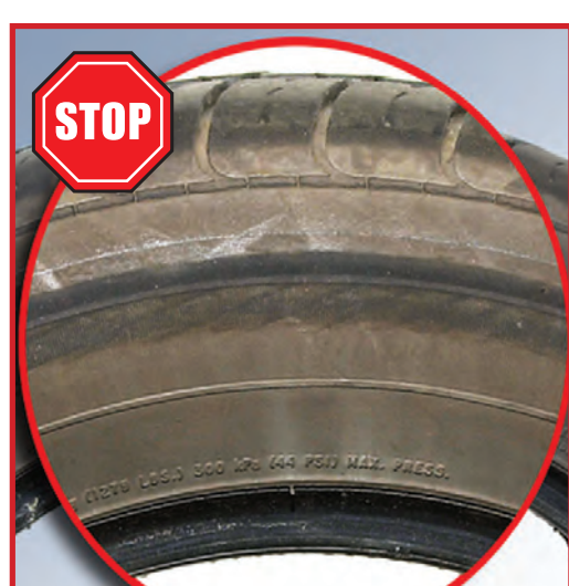
Heat Ring Excessive load/ Tire was run on flat
