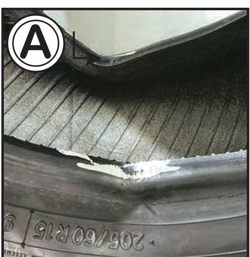
Kinked Bead Mishandling during shipping
