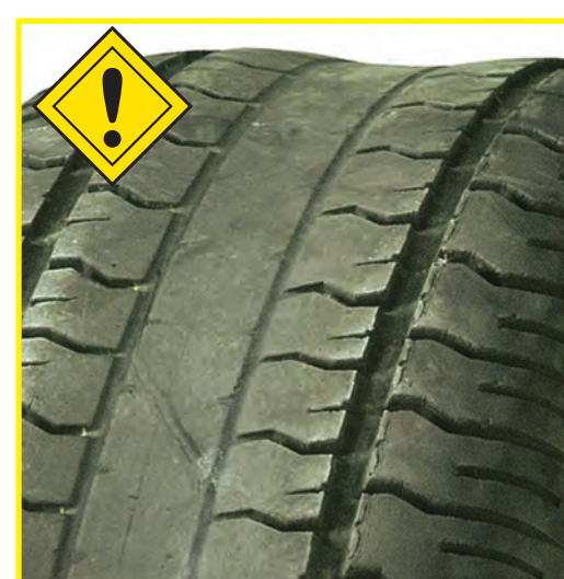
Center Wear Overinflation for load carried
