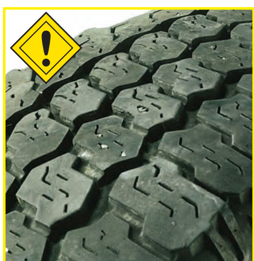
Irregular Wear Belt separation/ Worn suspension
