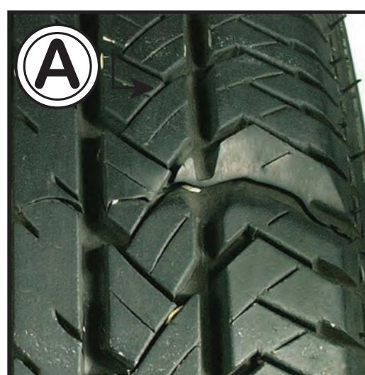
Open Tread Splice Underinflation/ Overloading
