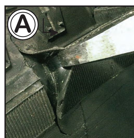
Sidewall Splice Underinflation/ Overloading
