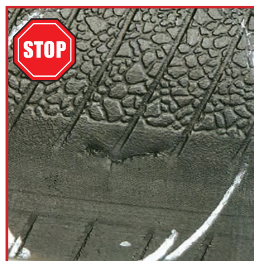
Impact Break Impact with object in road
