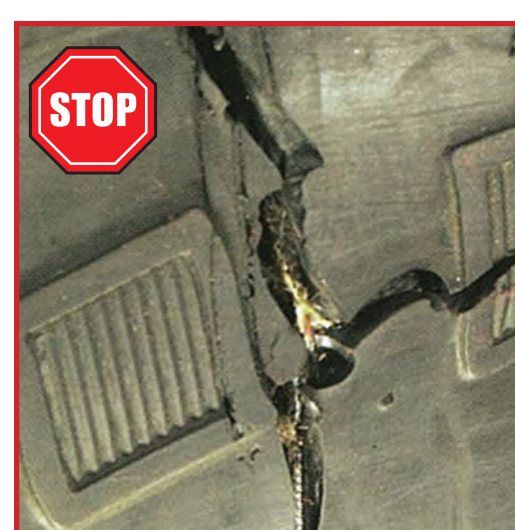
Sidewall Impact Break Impact with object in road
