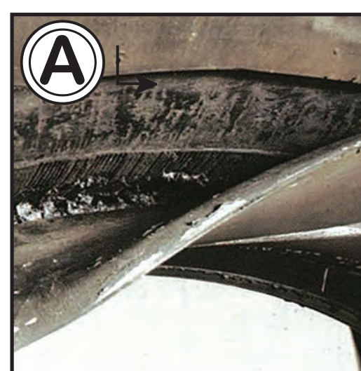
Bead Separation Excessive load/ Underinflation
