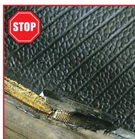
Mounting Damage Improper mounting procedures
