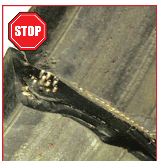
Broken Bead Improper mounting procedures
