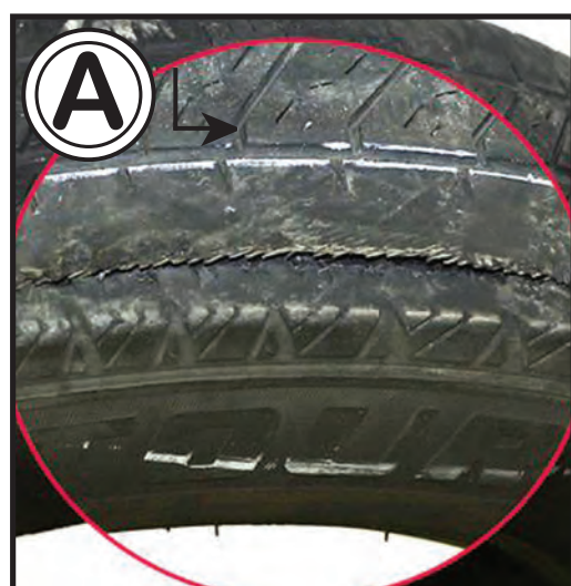
Belt Edge Separation Improper inflation/ Excessive load
