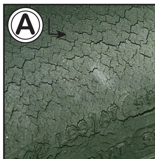
Ozone Cracking Exposure to sunlight/ Excessive heat
