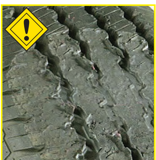
Flat Spot Brake lock/Skid
