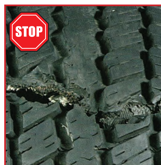
Impact Break Impact with object in road
