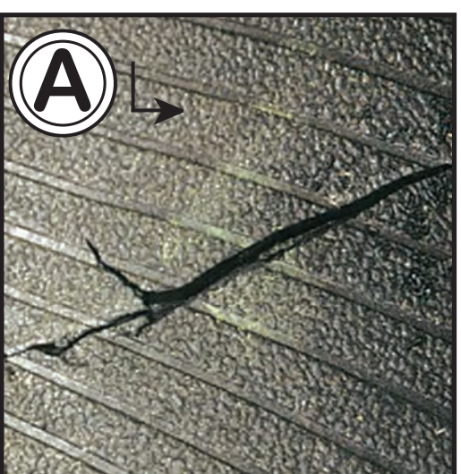
Liner Splice Tire was run on flat
