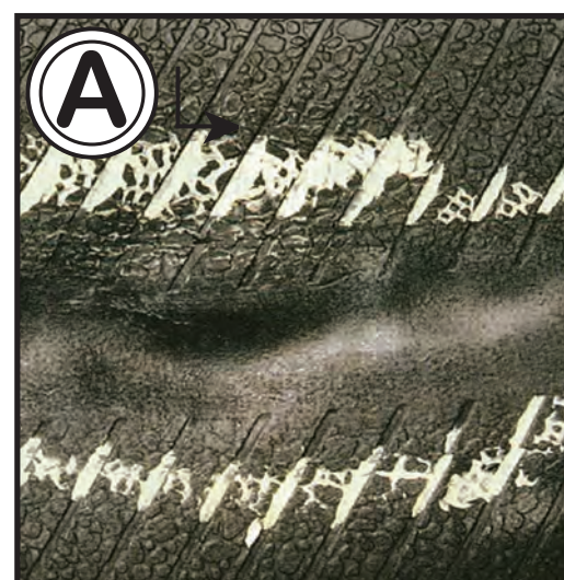
Blistered Liner Impact Damage
