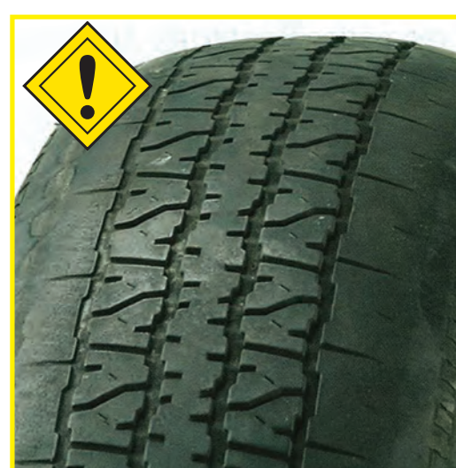
Underinflated Improper inflation pressure
