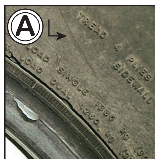
Bead Cracking Underinflation/ Overloading
