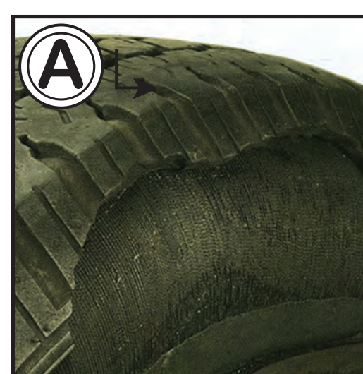
Sidewall Separation Impact damage/ Underinflation
