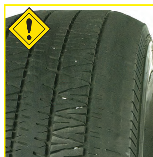
Alignment Wear Misalignment
