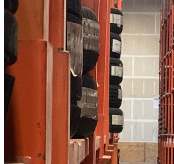
**Misaligned Racking.** Stand at the end of each aisle and look for any evidence of racks that are out of place or experiencing any sign of strain. Walk down each aisle and keep an eye peeled for any signs of damage.
