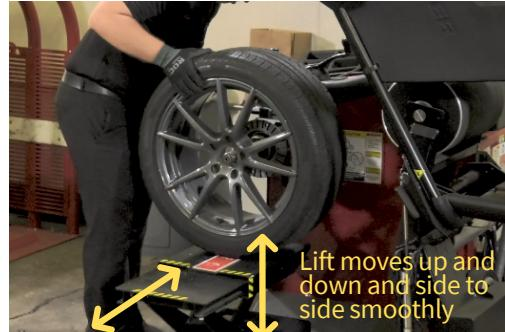
2. Is your balancer lift clear of debris under and around it?
