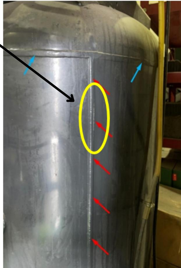
1. Spray the indicated welds with bubble check
