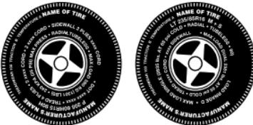
Shown here on the left is the sidewall of a popular 'P-metric' speed-rated auto tire. 'P' stands for passenger; '205' represents the width of the tire in millimeters; '60' is the ratio of height to width; 'H' is the speed rating; 'R' means radial; and '15' is the diameter of the wheel in inches. Some speed-rated tires carry a Service Description instead of showing the speed symbol in the size designation. The Service Description, 90H in this example, consists of the load index and speed symbol.
