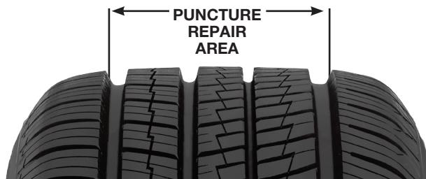
This graphic indicates that puncture repairs are limited to the tread area as generally depicted in the graphic. DO NOT make repairs where the injury damage extends into the shoulder/belt edge area OR where the injury extends at an angle into the shoulder area. If there is any question that the injury extends into the shoulder/belt edge area, then the tire must be scrapped.
