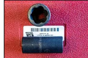
**Note:** If the wheel lock is stuck in the socket, partially thread the lock back onto the stud and move it side to side and up and down to remove it, using a torque stick for additional leverage, if needed.
