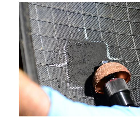
**10.** Use the contour rasp to buff the plug stem flush with the innerliner. Then, buff the area several times in one direction to get a patch area of about 3" x 3".
