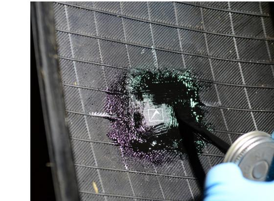
**16.** Apply repair sealer over the entire buffed area and the edges of the patch, leaving the center of the patch clear to expose the "Quality Checkmark."
