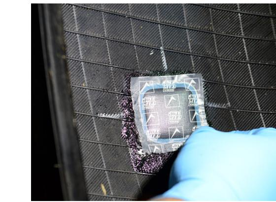
**14.** Firmly apply a universal patch by centering it over the plug stem.
