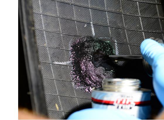
**13.** Apply a thin coat of quick dry patch cement to buffed area using a circular brushing pattern.
