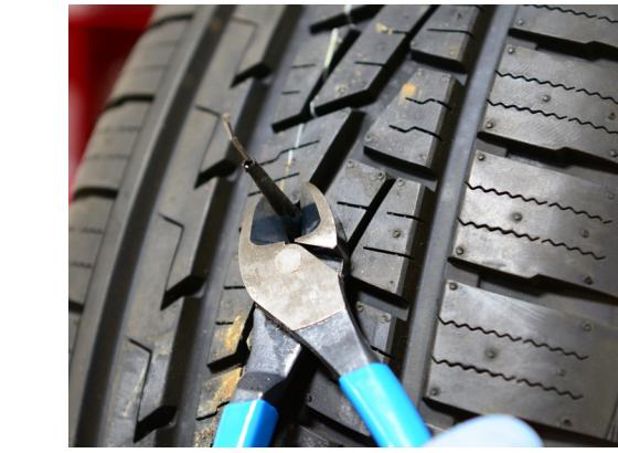
**17.** Use the diagonal cutters to cut the plug stem on the outside of the tire flush with the surface of the tread.
