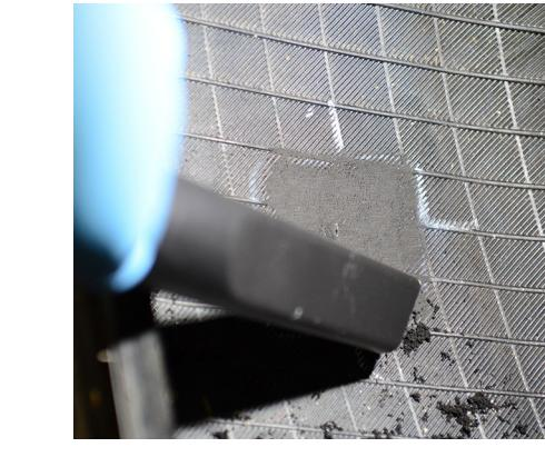
**12.** Use a vacuum to remove all debris from the inside of the tire.
