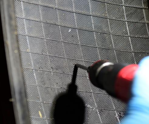
**5.** Use the carbide cutter to ream the injury **3-4 times from the outside in and inside out.**
