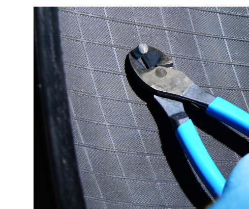
**9.** Use the diagonal cutter to cut the plug stem 1/8" above the innerliner.
