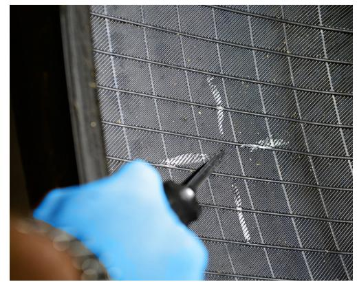
**2.** Inspect and probe the injury with an awl to determine the extent of the damage and the angle of the injury channel.
