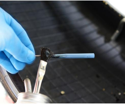
**7.** Fully coat the plug stem with quick dry patch cement.
