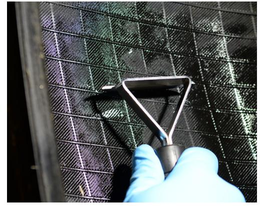
**4.** With the innerliner scraper, clean and scrape the injured area.
