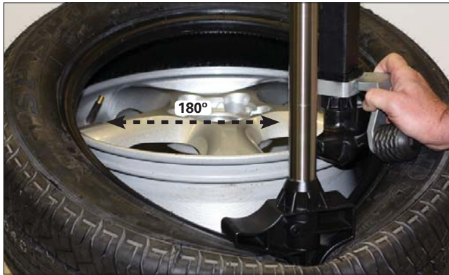
Figure 42 - Position Valve Stem 180° Ahead of Mount/Demount Tool
