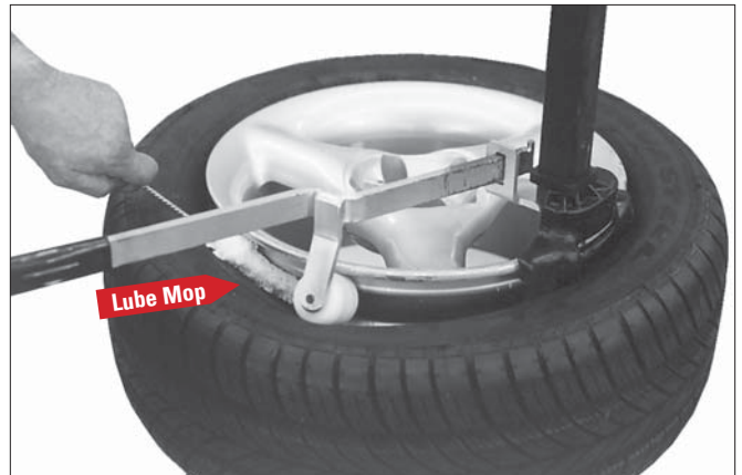
Figure 35 - Lubricate Upper Bead
