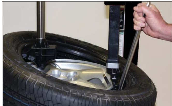
Figure 41 - Helper Holding the Lower Bead in Drop Center
