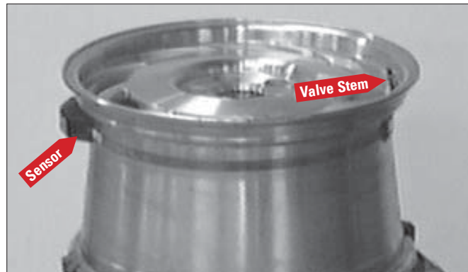
Figure 31 - Wheel with Low Pressure Sensor/Transmitter
