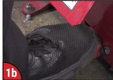
...and depress the blaster pedal **while Tech #2 inflates with the device outlined in the steps below.**
