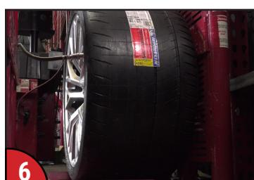
Remove the assembly from the tire changer and continue inflation inside of the cage using the approved inflation procedure.
