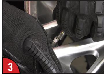
3 Feed the valve holder through the valve hole in the wheel and screw the valve into the valve holder.
