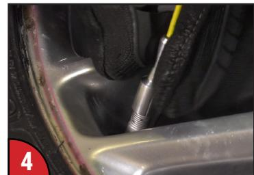
Remove the cable from the valve.
