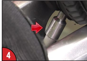
4 Note the orientation of the clocking indicator in relation to the TPMS sensor to ensure proper installation
