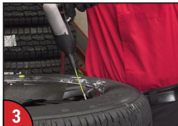
After inflation is complete, lift the tool from the wheel allowing the valve to seat into the valve opening.
