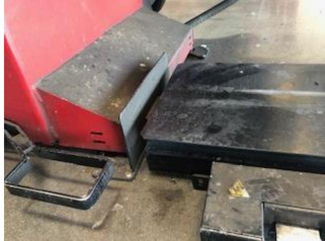
We have developed a new method of securing the balancer in place and keeping wheel weights from falling under the lift. This will help with weight chasing and costly repairs to the lifts. These attachments will not replace normal housekeeping. Please follow the guidelines for daily maintenance.
