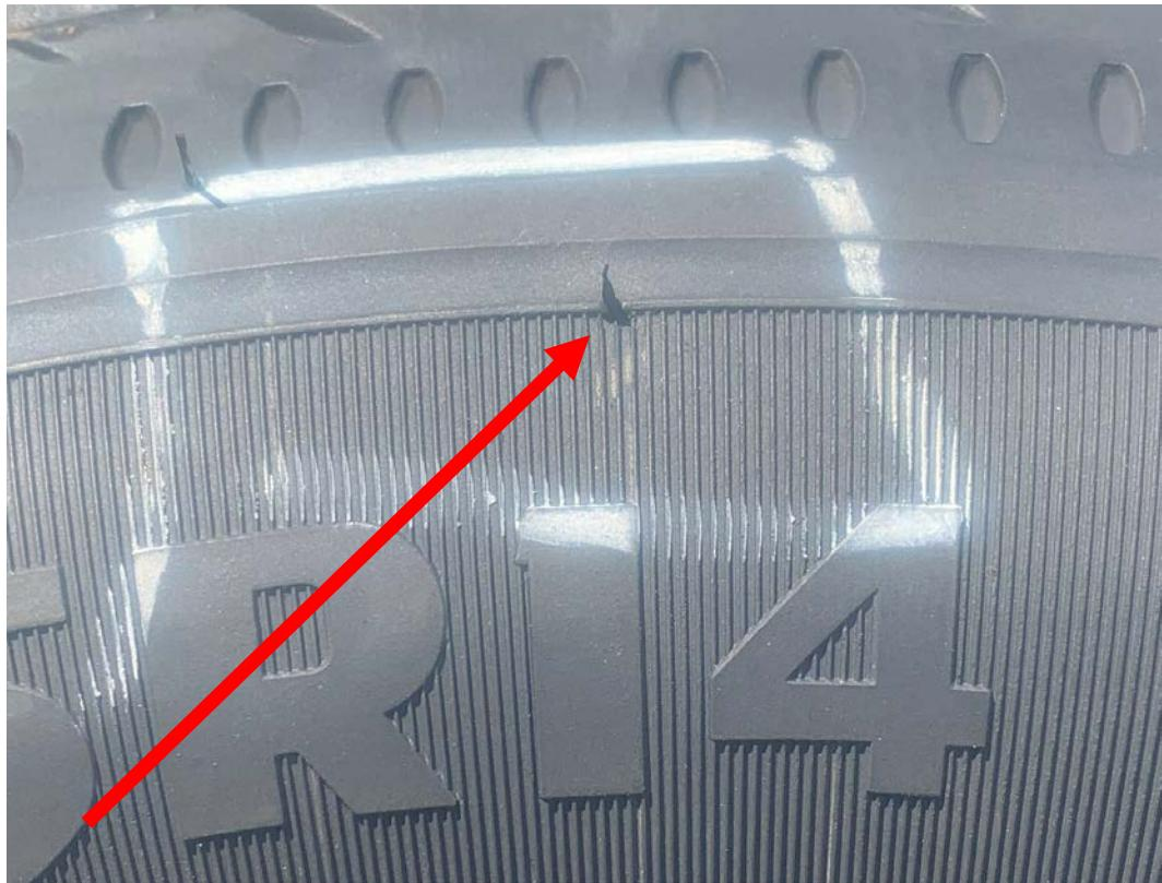
**REASON:** Some tires have been found with pinhole leaks in the upper sidewall.
