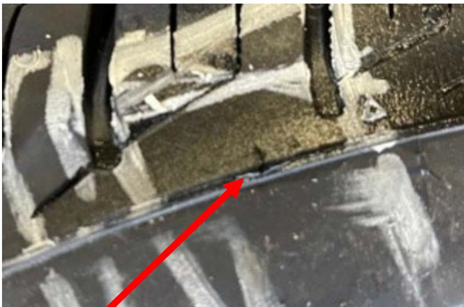
**REASON:** Some tires have been found with pinhole leaks in the upper sidewall.
