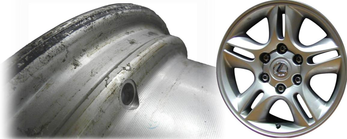
**The washer diameter on 7002A is 0.70in. Certain OE wheels have a valve hole counterbore diameter smaller than 0.70in. Retro-fit 7002A with 406K and install nut to 71 in-lbs.**
