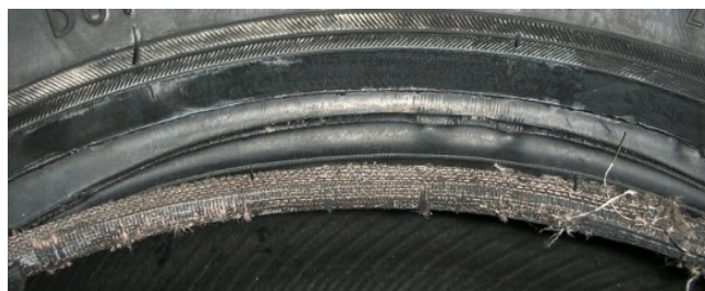
Damage to the bead from mounting
