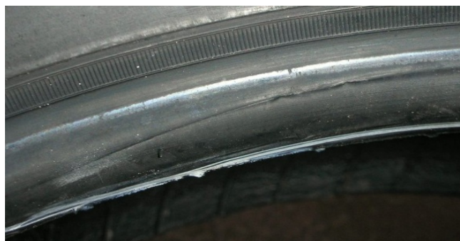
Damage to the bead from mounting
