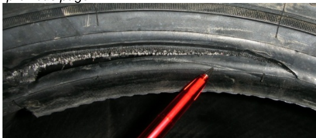
Damage to the bead from mounting
