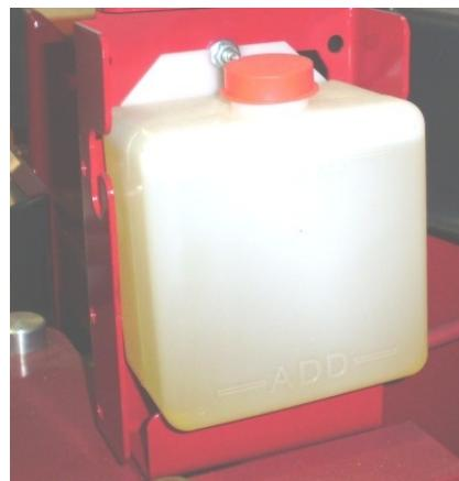
Inspect oil injector reservoir and fill as necessary with Coats oil pc.98303
