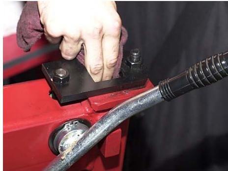
Clean the slide locking mechanism on top of the swing arm.
