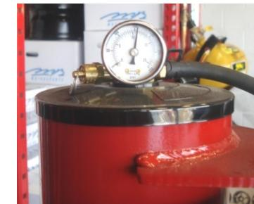
Confirm that the pressure gauge on the tower is functioning.
