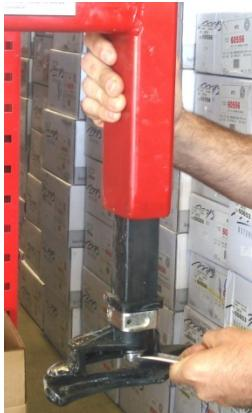
Remove the duck head and push the slide through the top of the swing arm.
