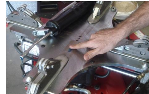
Lubricate the slide areas of the table top with a light coating of chassis grease.
