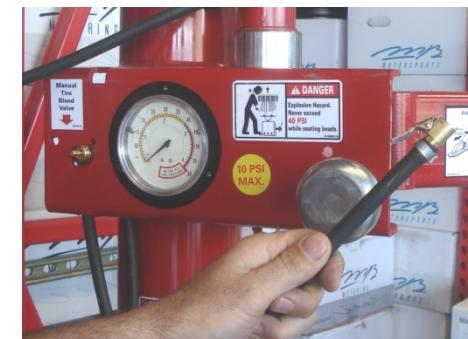
After the air is reconnected, hold inflation hose away from yourself and step on the pedal. A pulsing of air flow indicates that the 10psi limiter is working properly.
