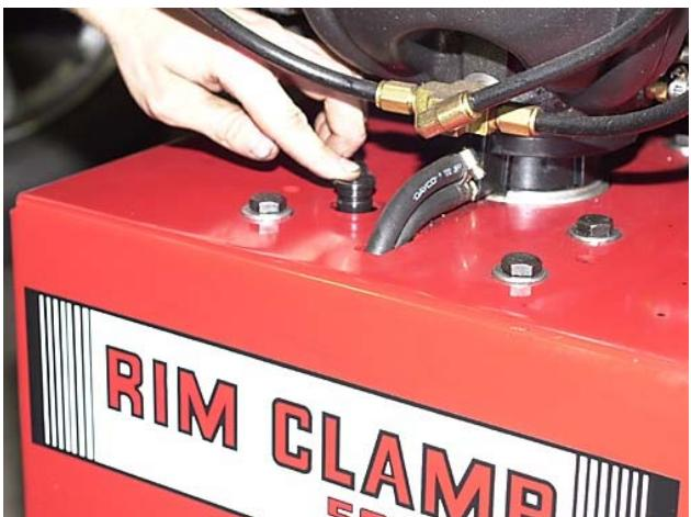
Check the fluid level in the transmission. If any fluid is visible on the dipstick, it is properly filled. If necessary, fill with SAE 75-90 gear lubricant.
